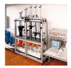
Every KRAL Volumeter® is calibrated on the in-house test rig. The measured values of this calibration can be traced back to «national normals». The reproducibility of the flow measurement is usually 0.01%.
